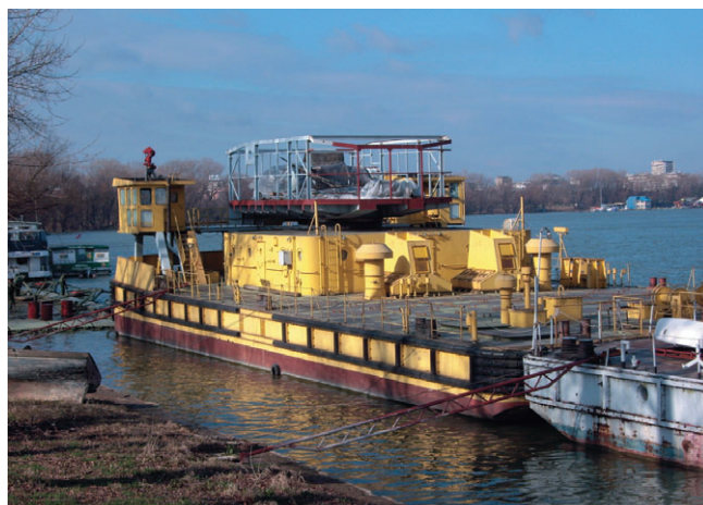
Slika 2 – Plovna dizalica LDI-500 u opremanju Figure 2 – Assembling of an LDI-500 floating crane
