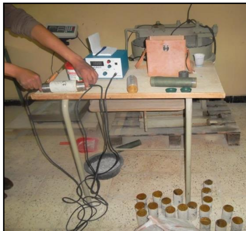
Figure 4 – Ultrasonic Pulse Velocity tests
