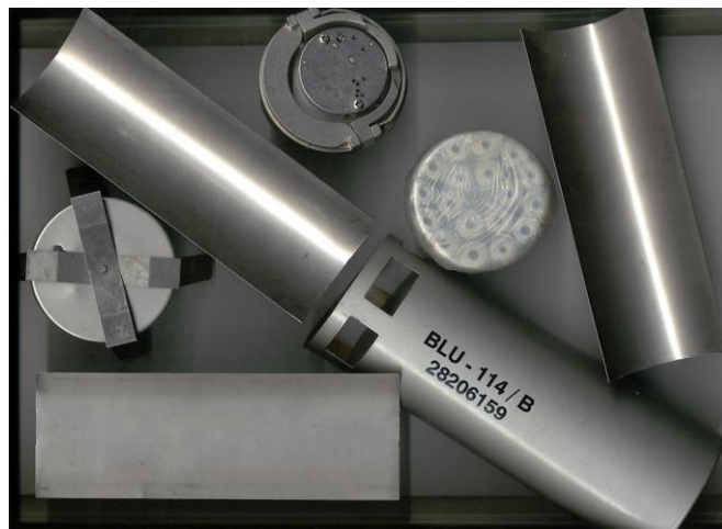
Figure 3 – Appearance of the cassette with threaded conductors
