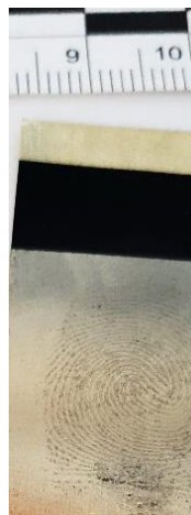
Figure 4 – Fingerprint on brass surface developed with the use of black magnetic fingerprint powder
