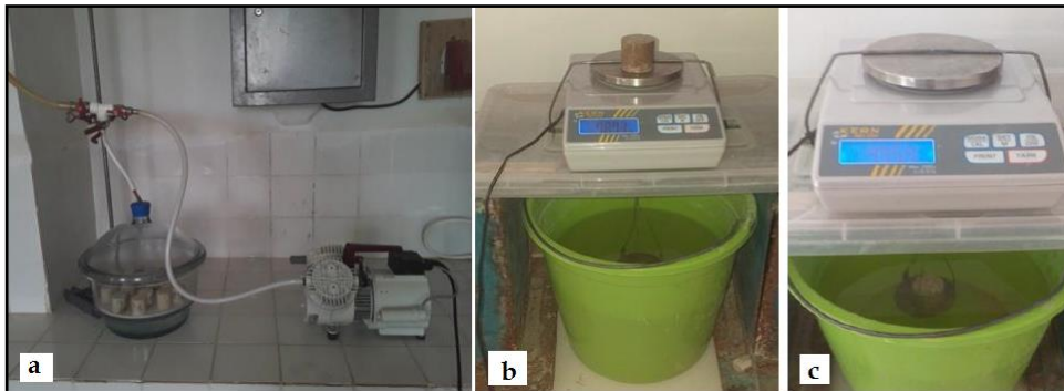
Figure 2 – Porosity tests: (a) vacuum saturation (b) weighed in air (c) hydrostatic weighing
