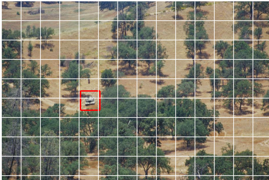
Figure 6 – Illustration of the principle of applying clutter metrics based on image quality assessment
