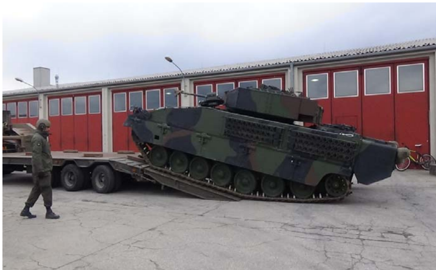
Figure 2 – Evacuation of a combat vehicle by a towing train
