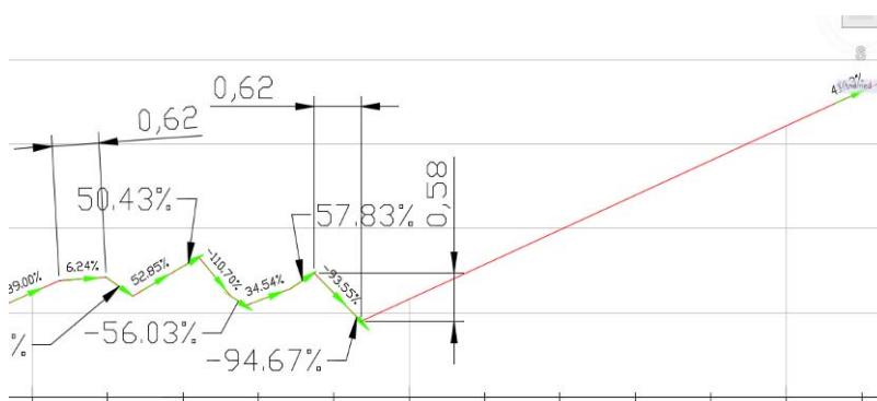
Figure 26 – Slopes of the surfaces shown on the transversal profile of the 3D surface model
