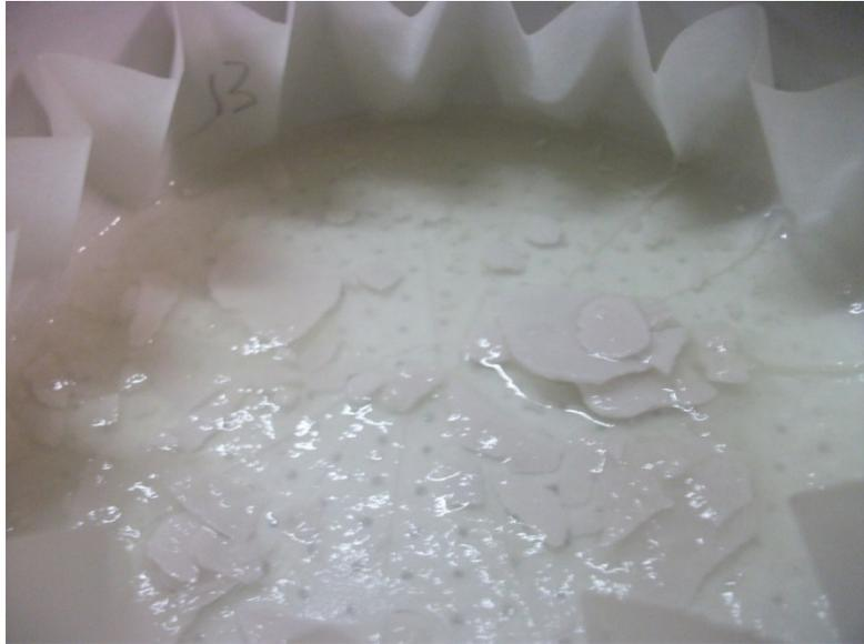
*Figure 4 – Typical gel formation in Experiment. 13*
