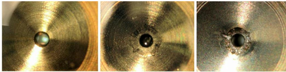
a b c Picture 7 – Look of the damaged nozzle (Common rail Injectors FAQ – triplet diesel injection – Waco, 2011)
