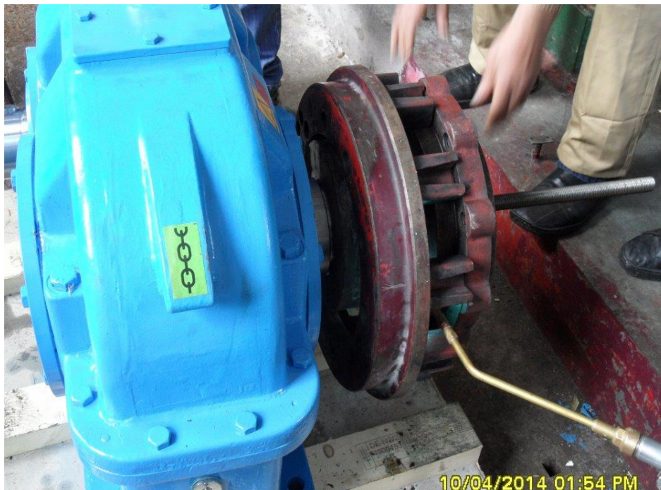
Figure 5 – High-quality installation of assemblies using the new device for dismantling and assembling
