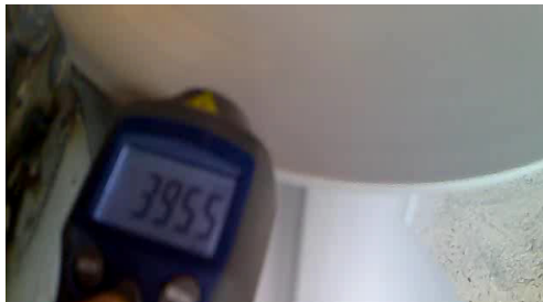
Figure 9 – Measurement of the number of rotor revolutions, where the vertical angle of the wind inlet is, in this case, increased for 15°
