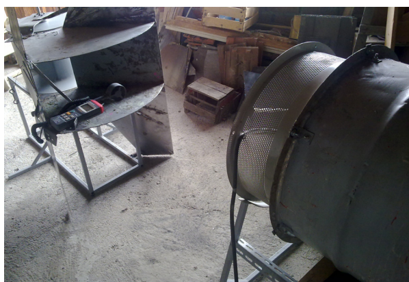
Figure 8 – The process of measuring the wind speed using an anemometer
