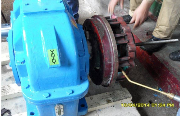
Figure 4 – Mounting of the metal parts of the elastic coupling N-EUPEX onto the multiplier assembly
