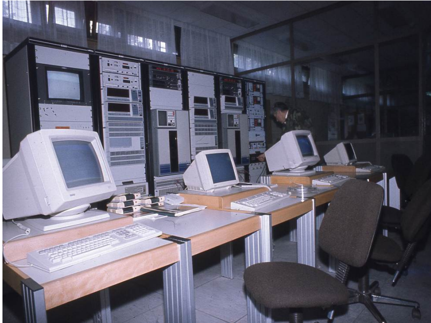
Figure 14 – Telemetry System PCM/FM, US company LOREAL - operator position, (Arhiv Vazduhoplovnog opitnog centra, 2016)
