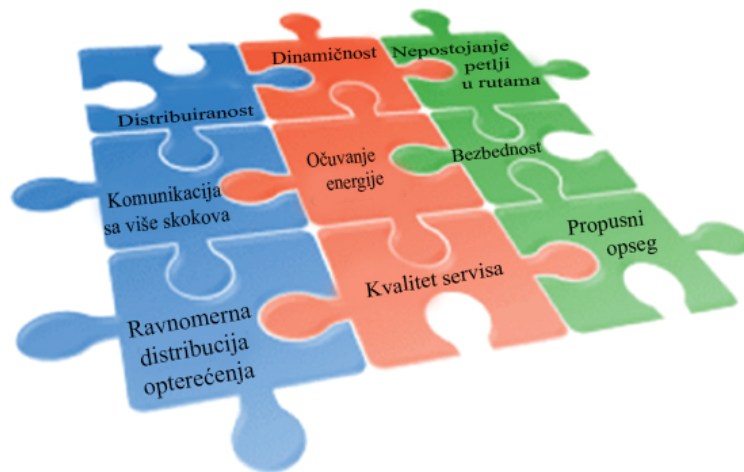
Slika 2 – Karakteristike protokola rutiranja u mobilnim ad hoc mrežama Figure 2 – Routing protocol characteristics in mobile ad hoc networks
